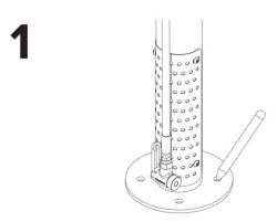
Place the Air Kit Prime in the desired location. Use a marker or pencil to outline the holes of the flange onto the base material.
