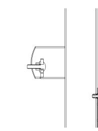
Firmly attach the carriage bolt to the pump with the nut and washer.
