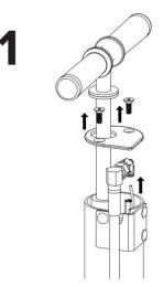
Remove the 2 tamper-proof screws at the top of the pump and lift the cap. Then disconnect the airline via the push-to connect fitting at the top of the hose.
