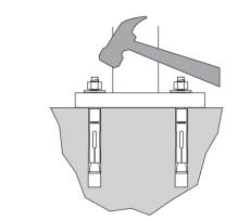
Thread nuts onto anchors, leaving approximately 1/4" of the anchor protruding, and tap into surface. Place the 2 provided tamper-proof penta nuts on opposite sides. Tighten nuts down to secure pump.
