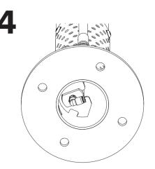
It may be necessary to gain access to the bottom of the main body to align the pump when reassembling.
