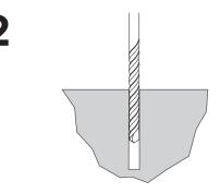
Drill the holes in accordance with the specifications shipped with the anchors. Make sure the holes are at least 3" away from any cracks in the base material.
