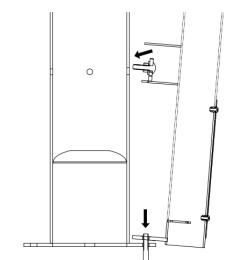
If attaching to a previously installed Fixit, remove the nut and washer on the wedge anchor on the side of the Fixit to receive the pump. Place the pump lower flange hole over the wedge anchor, and slot the previously attached carriage bolt through the hole on the side of the Fixit.
