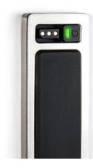
Assigned Use: User will be assigned a bike locker that will only work with a specific RFID key card. When these lockers are in use, there will be a green "In-Use" indicator light.
